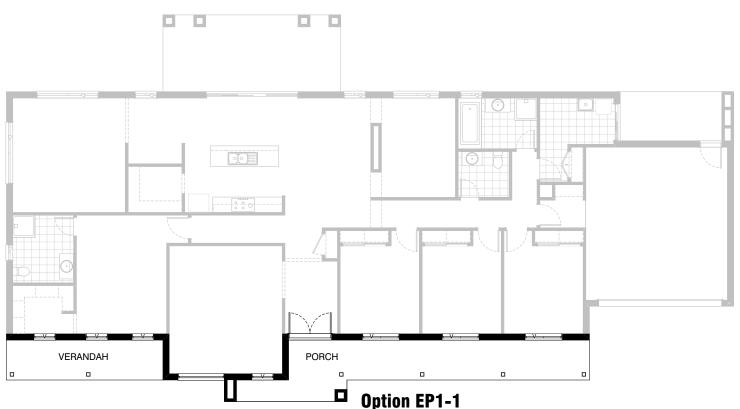
Provide Verandah to dwelling frontage including additional roof, structural concrete floor, 6no. 135mm x 135mm timber posts on stirups with painted finish, structural lintels and cement sheet ceiling lining with painted finish.
